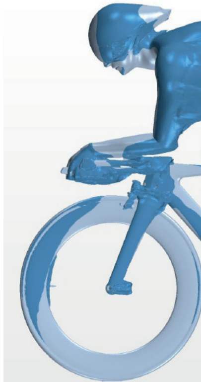
LOOK 596 – front brake and external steerer fork disturb the airflow
